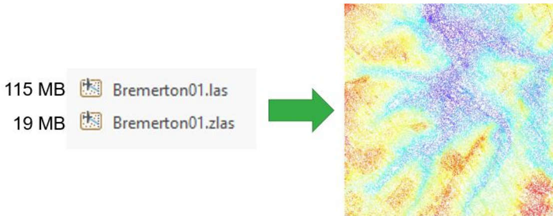
Figure 2.1. ZLAS files are compressed and optimized to perform better than raw LAS files.
