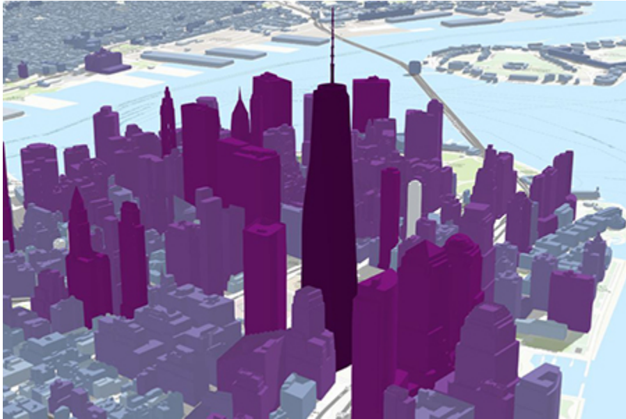
Figure 5.4. Multipatch features are enclosed volumes defined with three-dimensional rings and triangular patches. They are used to model the outer surface or shell of natural and as-built 3D features.
