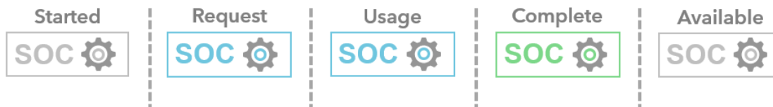
Figure 6.2. When a service instance is spun-up and started, it is ready to fulfill incoming requests from the client. When a request comes in, the ArcSOC responds to the request and sends the client back a result. When complete, the ArcSOC is released back into the pool and is ready to respond to additional requests.
