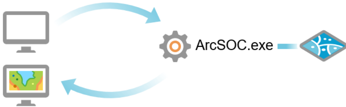
Figure 6.1. In this example, a map service has a single service instance, executed by an ArcSOC process, to fulfill requests made to the service. The ArcSOC process can respond to one request at a time.
