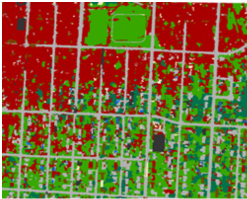
Figure 4.11. This damage-assessment map is a thematic raster created through semantic segmentation. (Data source: National Oceanic and Atmospheric Administration)
