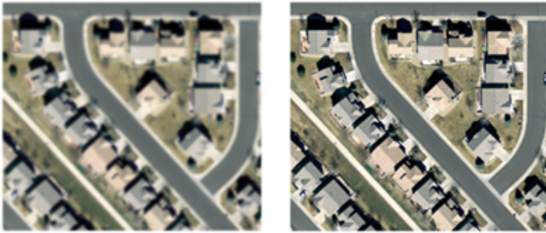
Figure 4.13. Image translation changed the low-resolution image on the left into the super-resolution image on the right.
