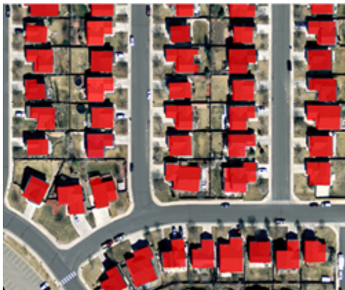
Figure 4.10. The boundaries of houses in this neighborhood were detected through instance segmentation.
