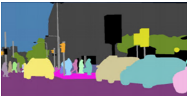
Figure 4.12. Panoptic segmentation of this street image classified each pixel and defined each unique object.
