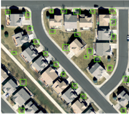
Figure 4.9. Trees in this neighborhood were identified from high-resolution imagery through object detection.
