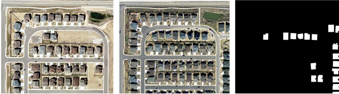
Figure 4.14. Houses built in the past five years were identified through change detection. (Data source: U.S. Geological Survey)
